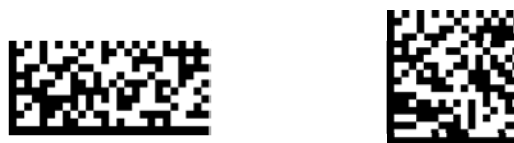
Fig. 7: Rectangular and square GS1 DataMatrix symbols (magnified symbols). The same data is encoded.
