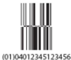
**Abbildung 3: GS1 DataBar Stacked Omnidirectional**
