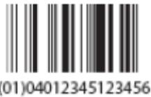
**Abbildung 1: GS1 DataBar Omnidirectional**
