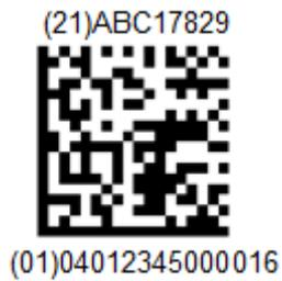
Figure A3: Direct marking of a supply item with GS1 data matrix
