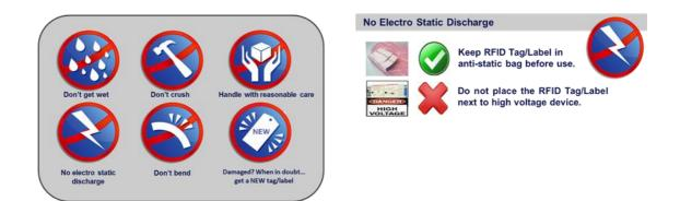
Another source of trouble for the functioning of an RFID tag consists in **water contact** and exposure to **high electric discharge**. In this context, washable RFID tags are usually encapsulated appropriately to prevent them from being destroyed by water contact. An RFID tag supplier can provide more information on the suitability of distinct tags. Last but not least, RFID tags/labels should not be attached directly on top of each other.
