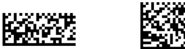
Fig. 5-2: Rectangular and square (GS1) data matrix symbol. Both symbols contain the same data.
